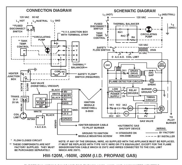
ELECTRICAL WIRING DIAGRAMS FOR THE HW-120M, 160M, AND 200M WATER HEATERS I.I.D. SYSTEM (PROPANE)
